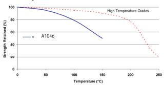
"Hot strength" shear strength tests performed on mild steel. 24hr cure at room temperature and conditioned to pull temperature for 30 minutes before testina
