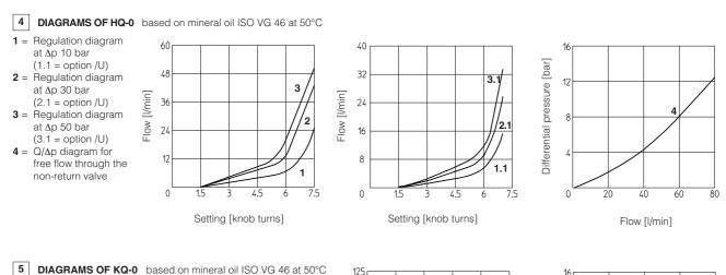
5 DIAGRAMS OF KQ-0 based on mineral oil ISO VG 46 at 50°C
