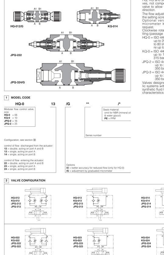
HQ, KQ and JPQ are flow throttling valves, not compensated, and with check valve to allow free flow in the opposite direction.
