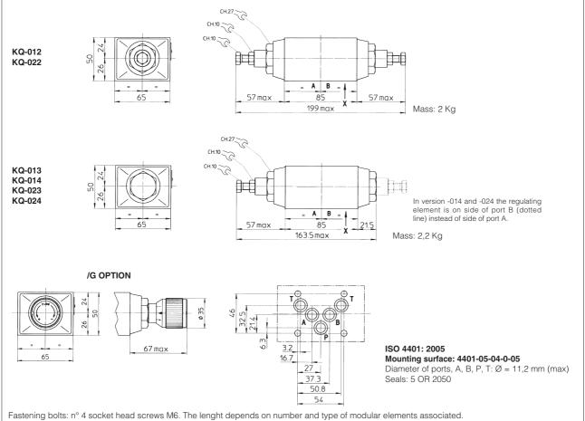
10 INSTALLATION DIMENSIONS OF JPQ-2 VALVES [mm]
