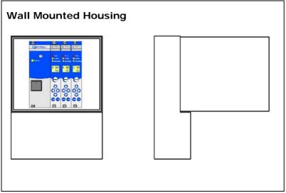
The wall mounted housing can be mixed with level swiches for GM Detector and for Nal Detector. The wall mounted housing has a back plane. Up to 3 Mini Switch units can be installed.
