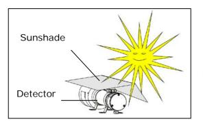
Direct insolation is not permitted. Otherwise, you have to install a sunshade in order to avoid a head up of the detector
