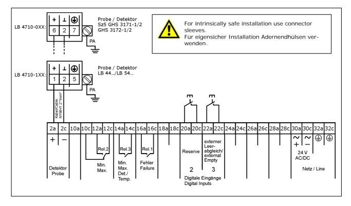
*Figure 5: Connection diagram of frame connector*
