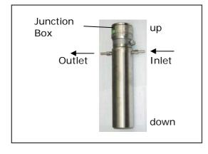
If the detector is installed vertically, then the connection pieces have to be on top.
