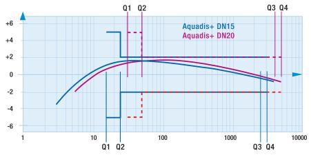
The dynamic range is defined as the Ratio (R) between the Nominal and the minimum flowrates. The MID approval proves the Aquadis+ real capacity to withstands to higher nominal flows (Q3 > Qn).
