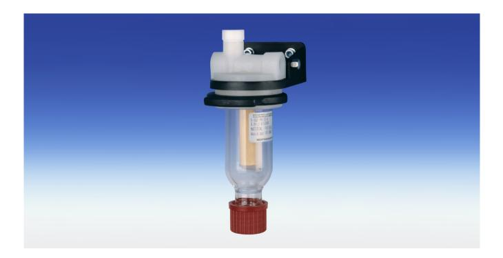
The removal of aerosols from sample gas streams is a requirement in many applications. To meet this need, the Bühler Model K-AGF-PV-30-A filter makes use of a coalescing element made of borosilicate fibers. The gas stream passes through the element from inside to outside. The aerosols are caught in the matrix forming steadily growing droplets which eventually drop into the bowl as a liquid. The liquid collected in the bowl is drained off by either by a condensate drain or peristaltic pump.
